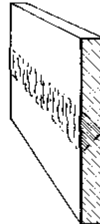
Horizontal position groove weld (2 G)
