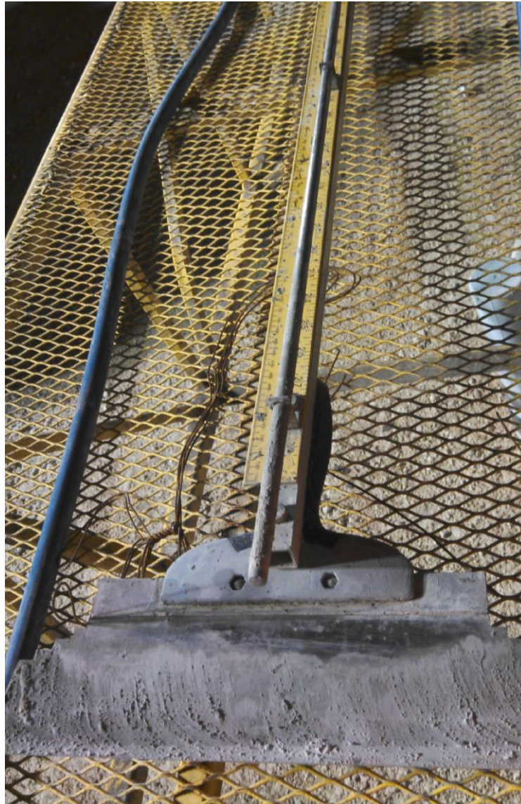
Homemade Rebar Cover and Slab Depth Check Gauge
