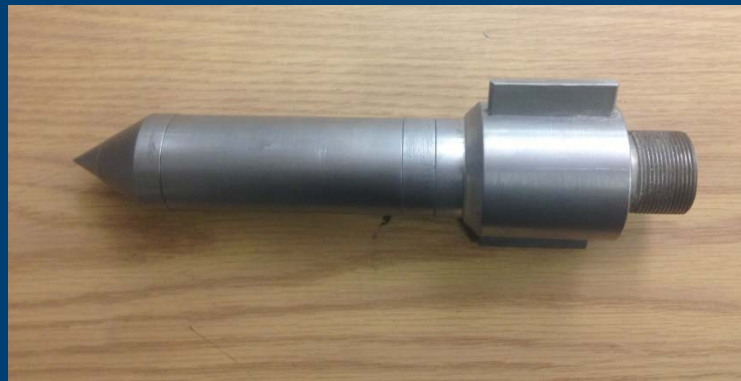
Vertical Insitu Permeability (VIP) Probe
