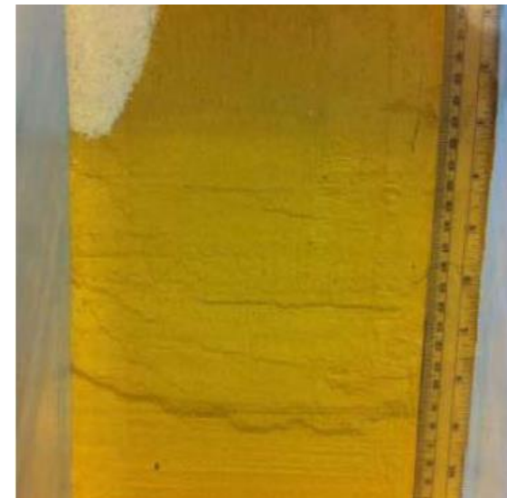
Observed rupture on surface of embankment in Test 10
