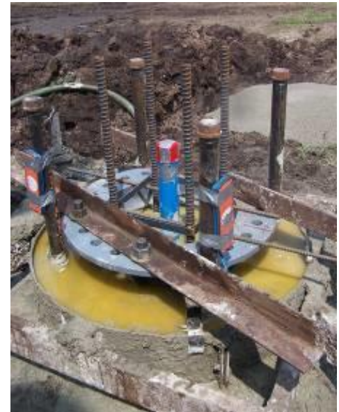
Pipe and flange connector (for combined torsion and lateral loading)
