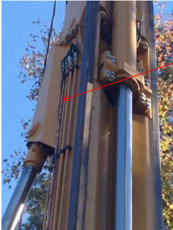
Cabling secured to Hydraulic lines
