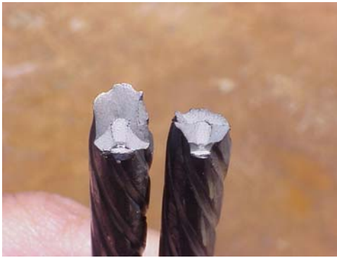
Figure 9 – Close-up View of Failure Plane Showing Depth of Heat Penetration
