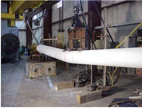
Figure 17 – Splice Test Specimen Under Load
