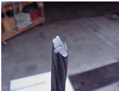
Figure 7 – Fracture Through Weld
