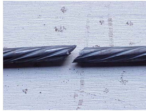
Figure 10 – Angled Fracture of Bar
