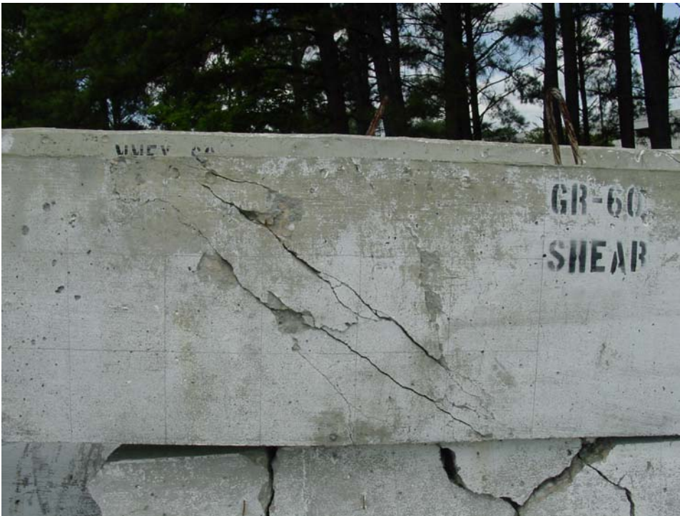
Fig. 12 Grade 60 Test 4 Beam
