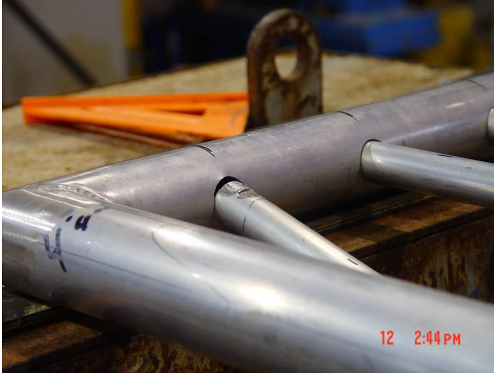
Figure 4: Slipping of Non-welded End
