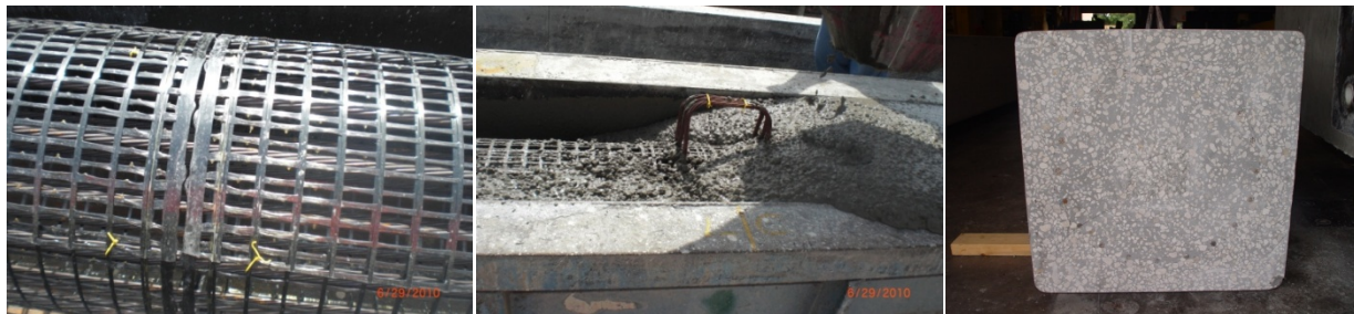
Figure 2 – CFRP mesh in casting bed at butt joint (Left). CFRP Mesh during concrete pour (Middle). Pile section (Right).
