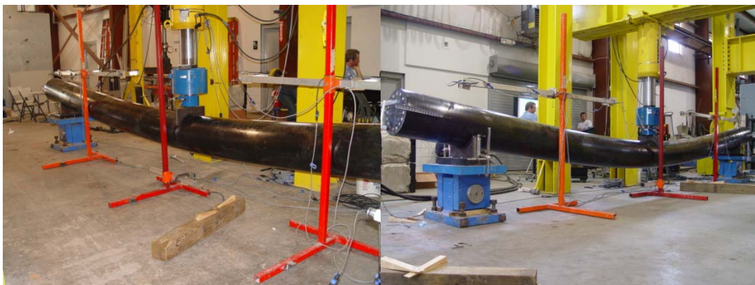
Figure 16: Testing a CP Specimen
