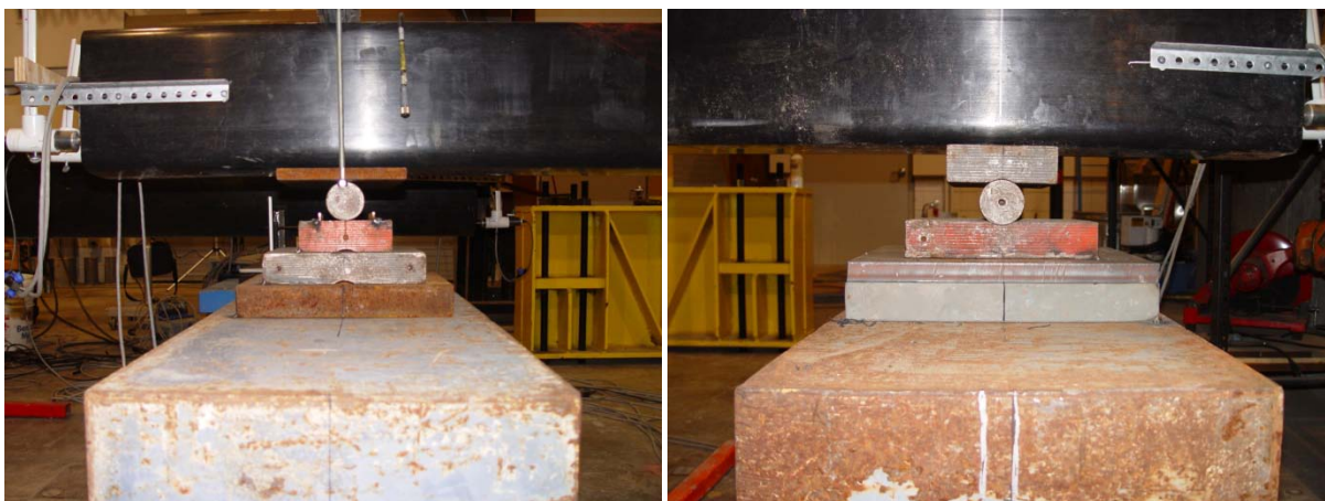
Figure 5: North Roller Support (left) and South Rocker Support (Right) for SCL Test Setup
