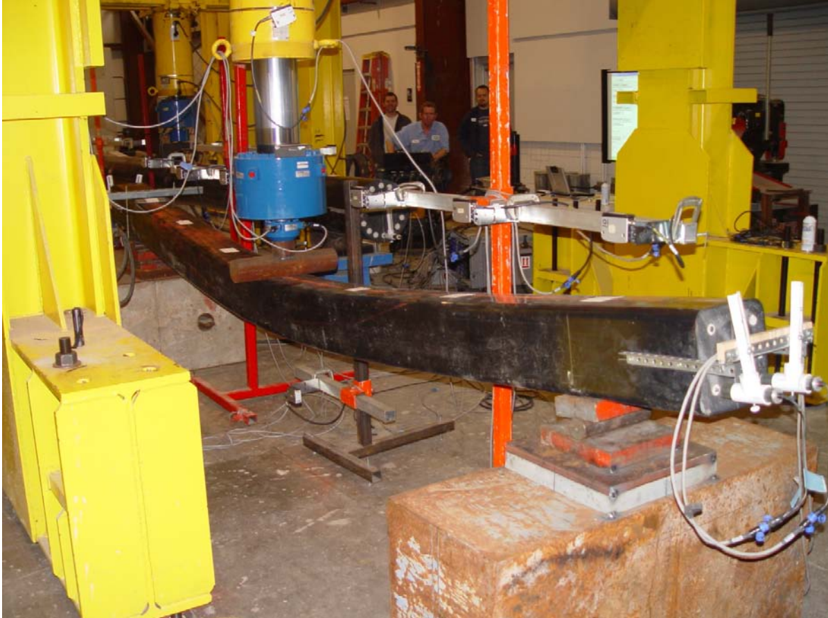
Figure 1: 3-Point Loading Test of a SCL Wale
