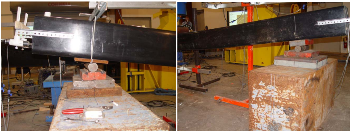
Figure 7: North Roller Support and South Rocker Support during Testing
