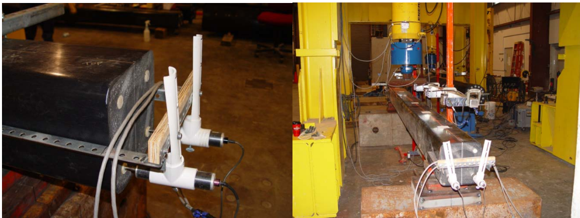
Figure 11: Deflection Gauge Setup for Detecting Slip of Reinforcement for SCL Specimens
