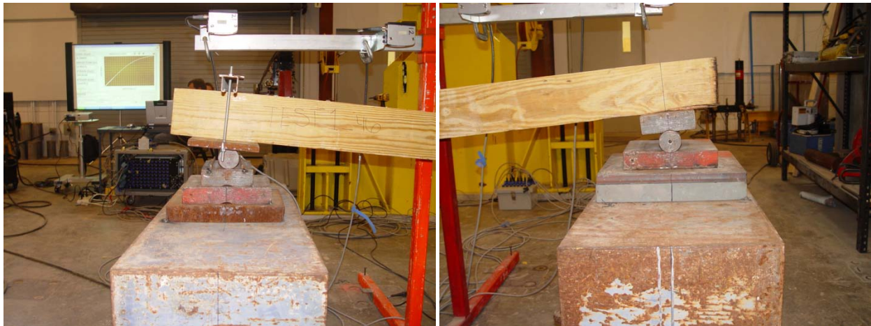
Figure 3: North Roller Support (left) and South Rocker Support (right)
