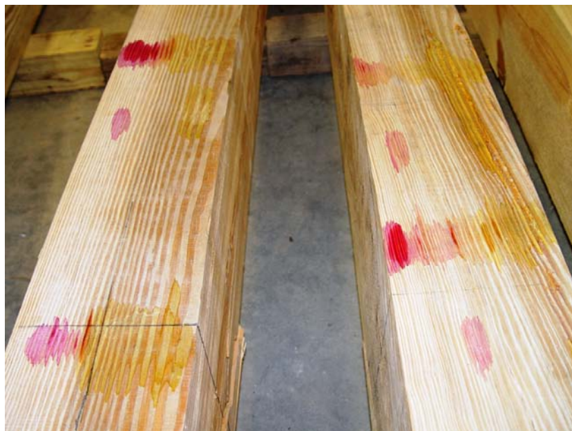
Figure 18: Variable Phenol Red Results: TimberSIL (left), Control (Right)
