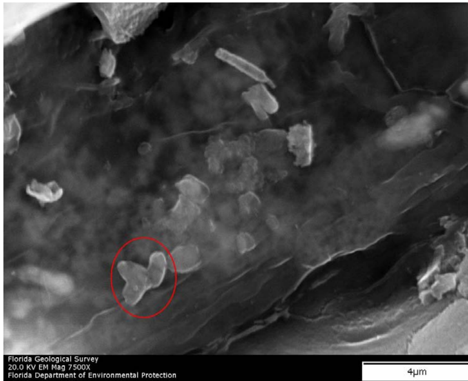
Figure 23: Microscopic Quartz Crystal in between Wood Fibers
