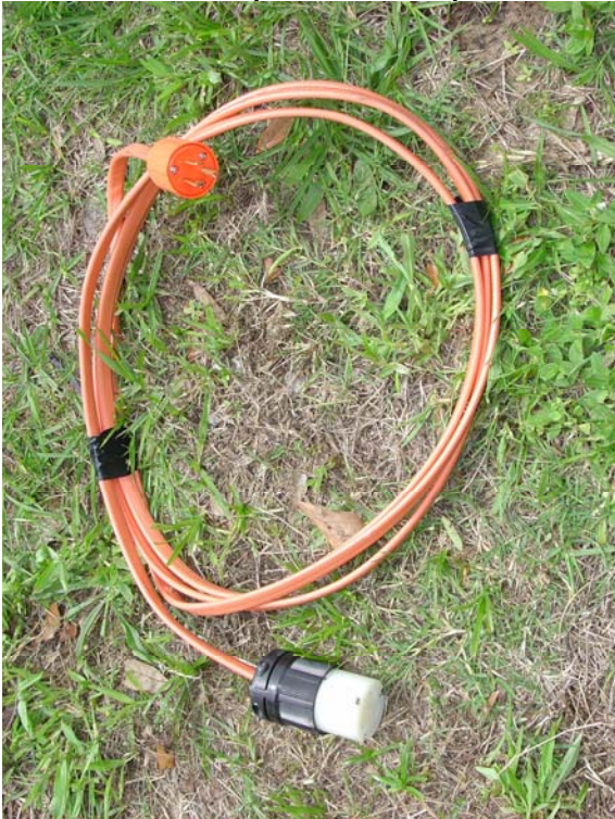
Generator Cable Twist Lock Connector can be secured to transfer switch with pad lock.
