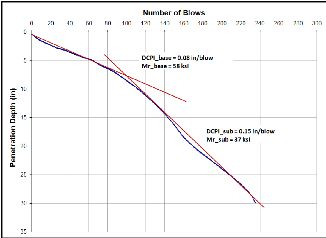
Figure B13. DCP Data Analysis on Section 50020000-2A.
