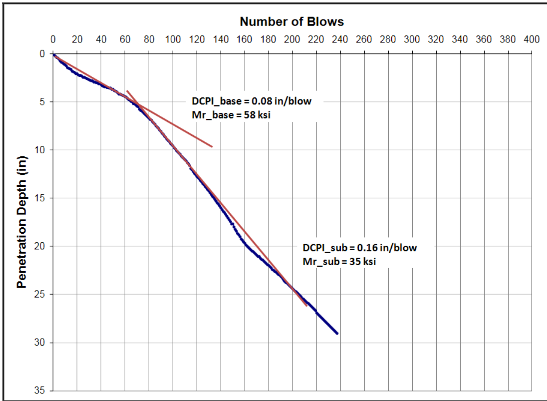
Figure B25. DCP Data Analysis on Section 77002000-2A.
