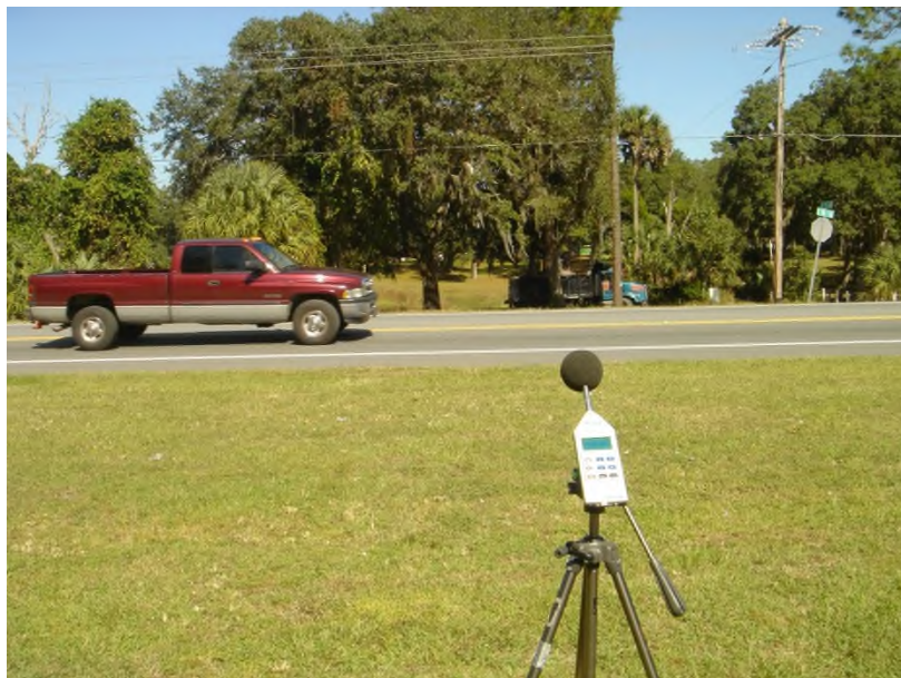
Figure 15. Nearby Passby Microphone Location During Tire/Pavement Test
