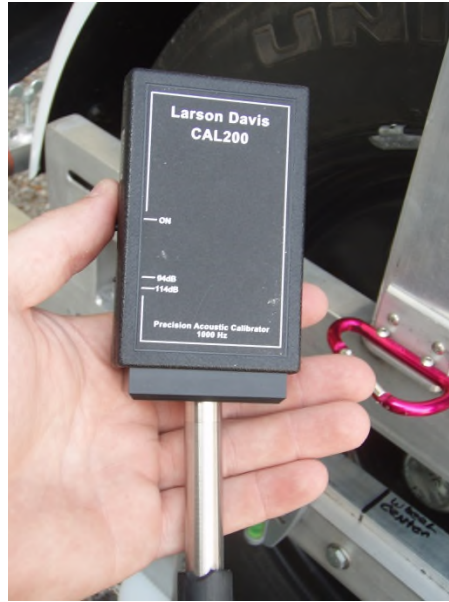
Figure A.1.13. Sound pressure calibrator applied to end of microphone/preamp combination, a switch is visible that adjusts the calibrator from a 94 dB tone to a 114 dB tone, this is to be set to 94 dB
