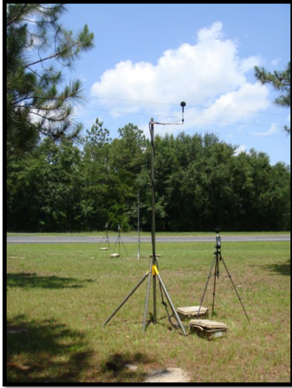
Figure 14. Typical Passby Equipment Configuration (sound level analyzers at five and twelve feet above pavement [Nearby meteorological station is not shown.]
