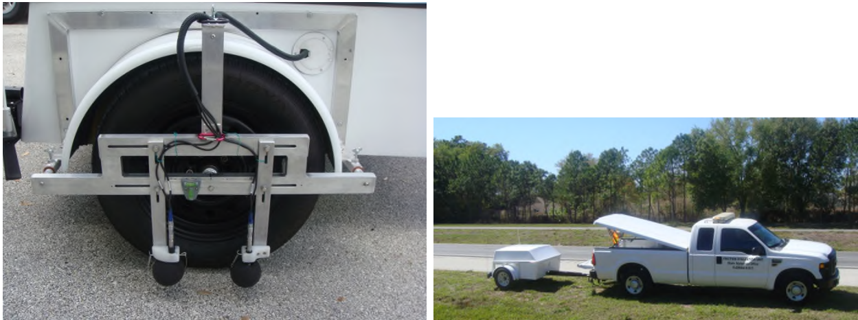
Figure 7. Final Rig, Intensity Probes, and Overall Vehicle System, Phase 2
