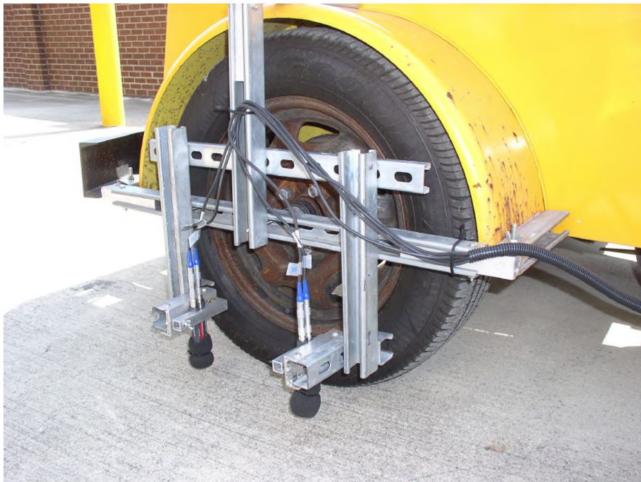
Figure 1. Prototype Test Rig With Intensity Probes, Phase 1
