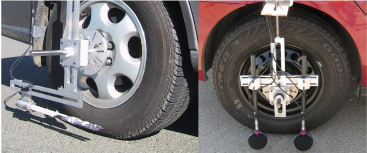
a. Horizontal configuration (single probe) b. Vertical configuration (dual probe)
