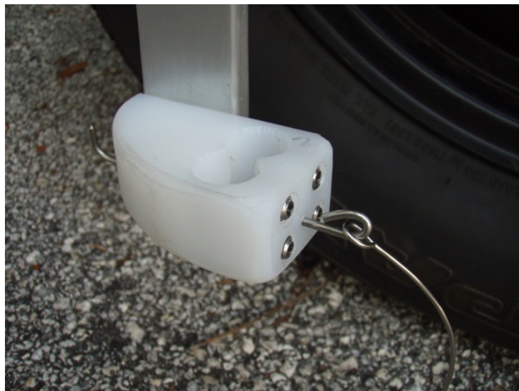
Figure A.1.16. Nylon mounting brackets for the microphone/preamplifier assembly
