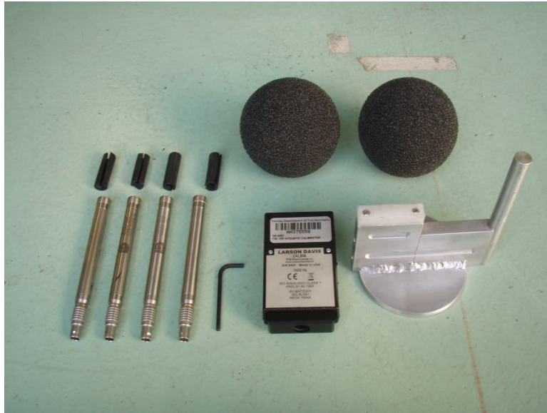
Figure A.1.10. Microphone/preamplifiers (previously attached), neoprene inserts, allen wrench, calibrator, windscreens, windscreens, and probe location tool.
