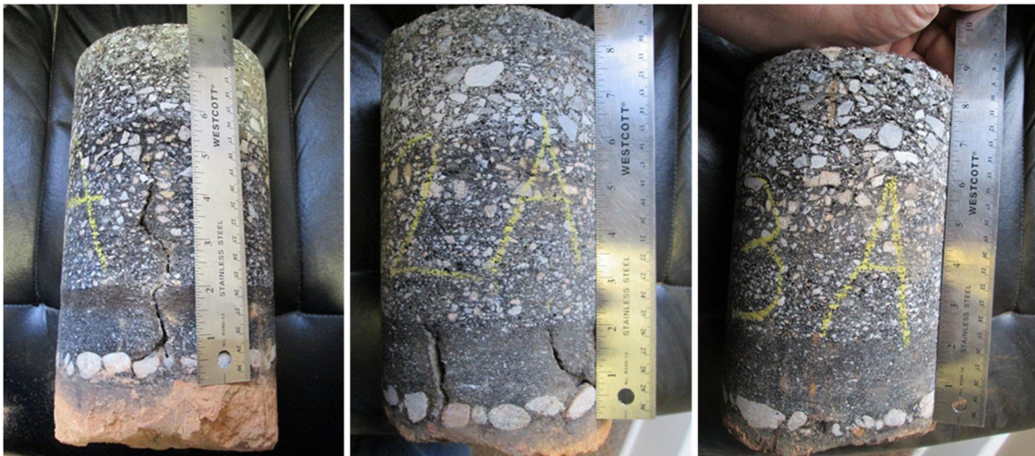
Figure 69: Core samples extracted over the Site 1 (Gulf County, SR 22) Pavement section.
