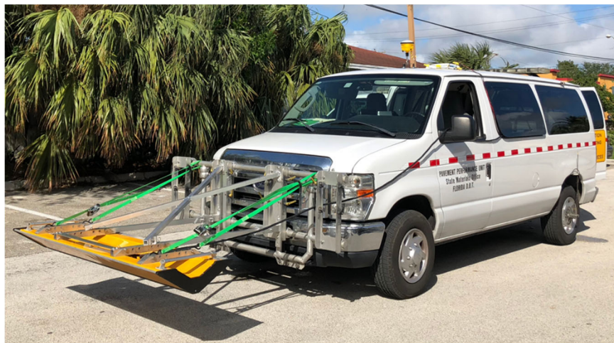
Figure 2: 3D-Radar test vehicle employed for Stage 2 data collection.
