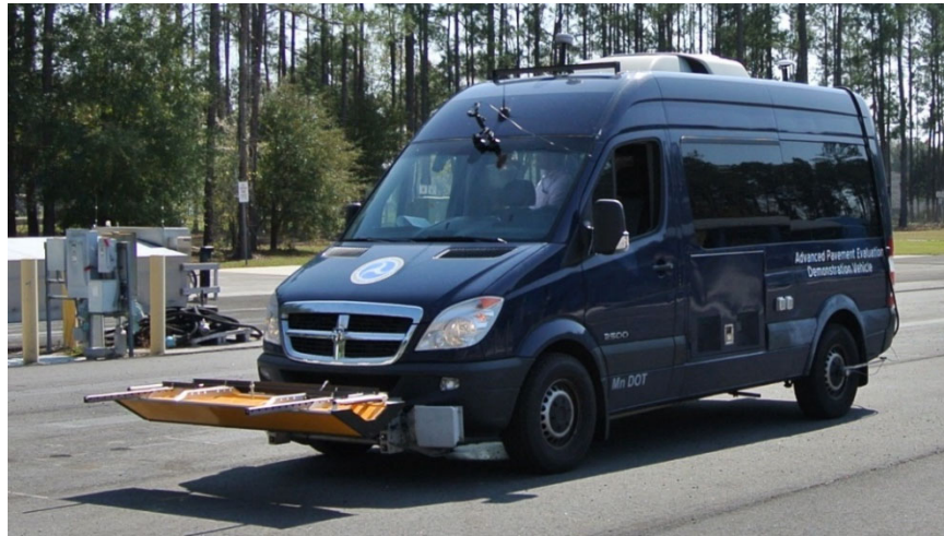
Figure 1: 3D-Radar test vehicle employed for Stage 1 data collection.
