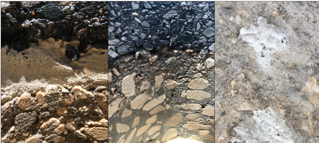
Figure 12: Examples of unidentified clay-type slurry, revealed after the milling procedure.
