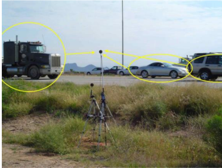
Figure 19. CTIM measurement setup (Lodico and Donovan, 2018)
