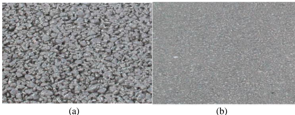
Figure 27. Surface texture of (a) porous asphalt; (b) dense asphalt (EAPA, 2007)
