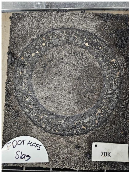
Figure 23: Failed HFCS Slab with Slag Aggregate
