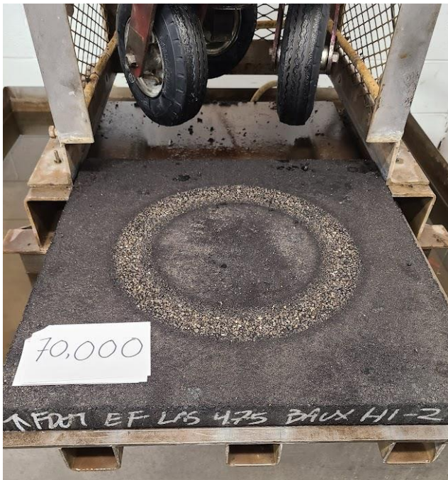
Figure 21: Slab after Polishing
