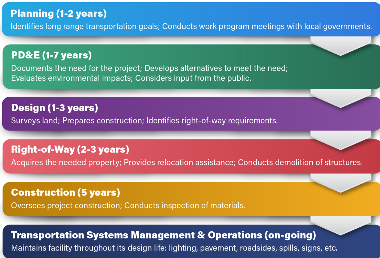
Figure 7. Overview of Project Development Cycle and Phases
