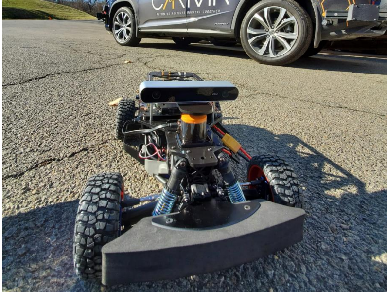
Figure 4. One-tenth scaled-down physical vehicle (CARMA 1/10th). Source: FHWA
