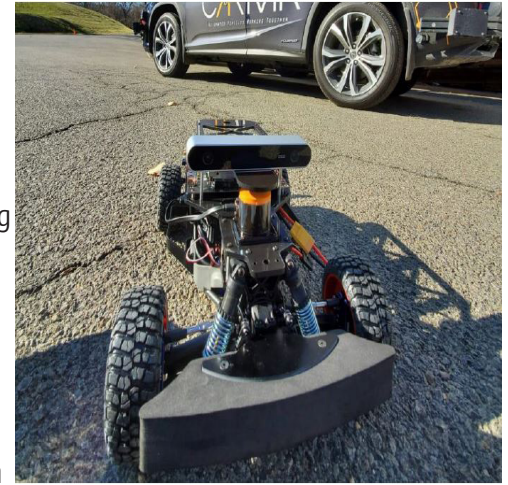
This project deployed a physical cooperative driving automation (CDA) vehicle, the CARMA 1Tenth, on a facility at SunTrax test track. Image source: FHWA
