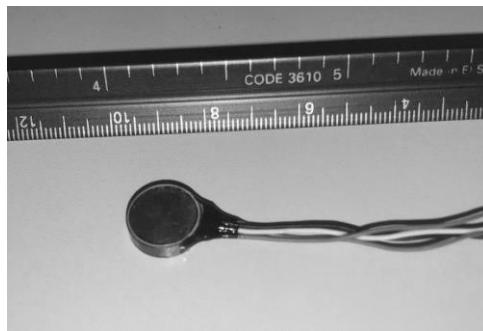
Figure 3-25. Pressure sensor used in centrifuge tests
