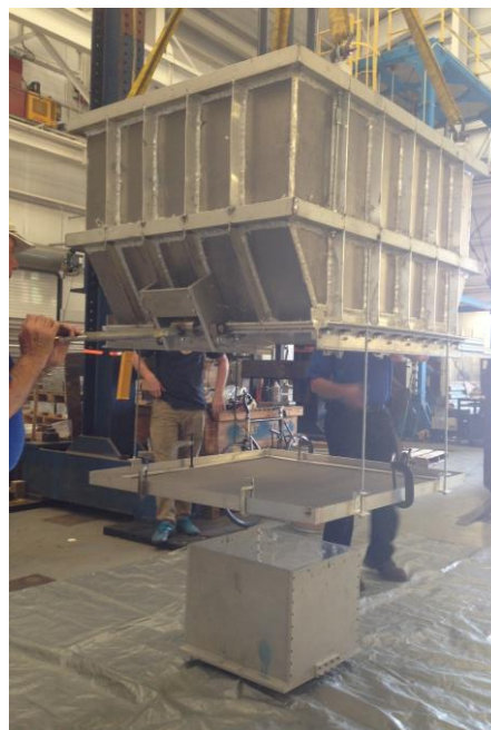
Figure 3-14. Pluviator used for constructing the soil profile
