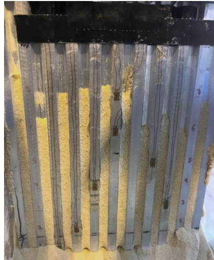
Figure 3-47. Soil plugging observed in centrifuge tests
