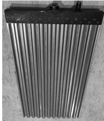
Figure 3-36. Helmet fixed to the model sheet pile wall
