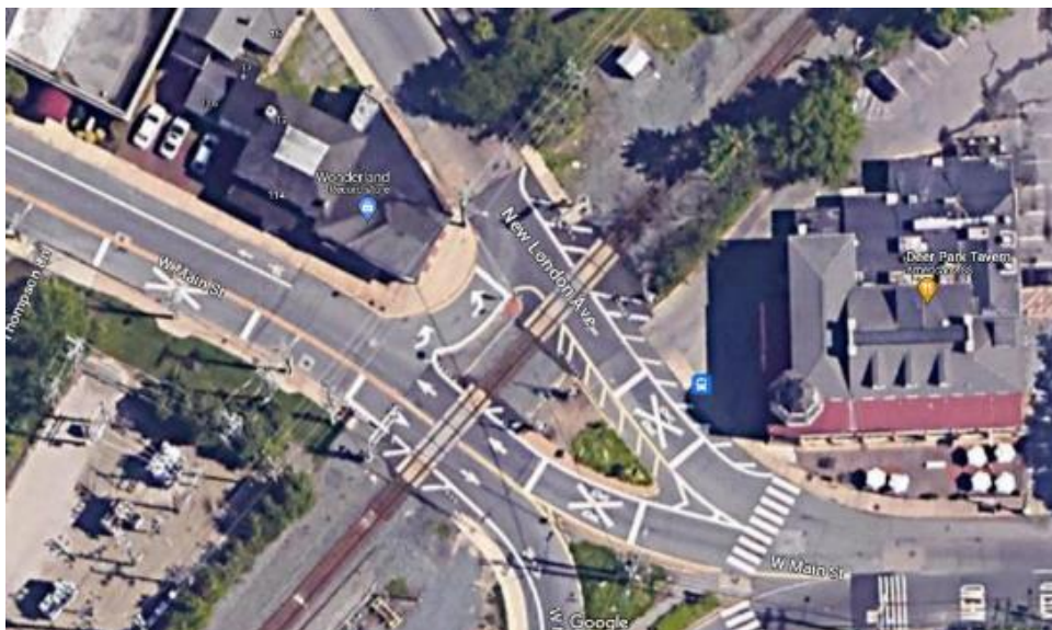
Figure 5-11. A Successful Delineator Deployment at an HRGC in Newark, Delaware
