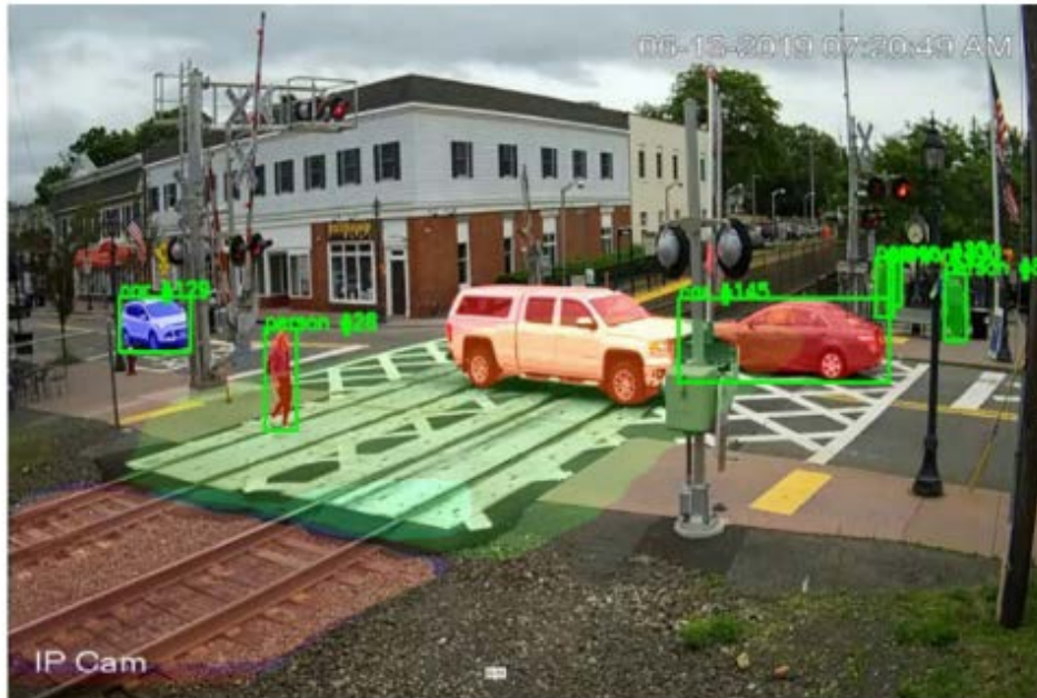
Figure 2-9. Example of an Automated Video Processing at an HRGC (64)
