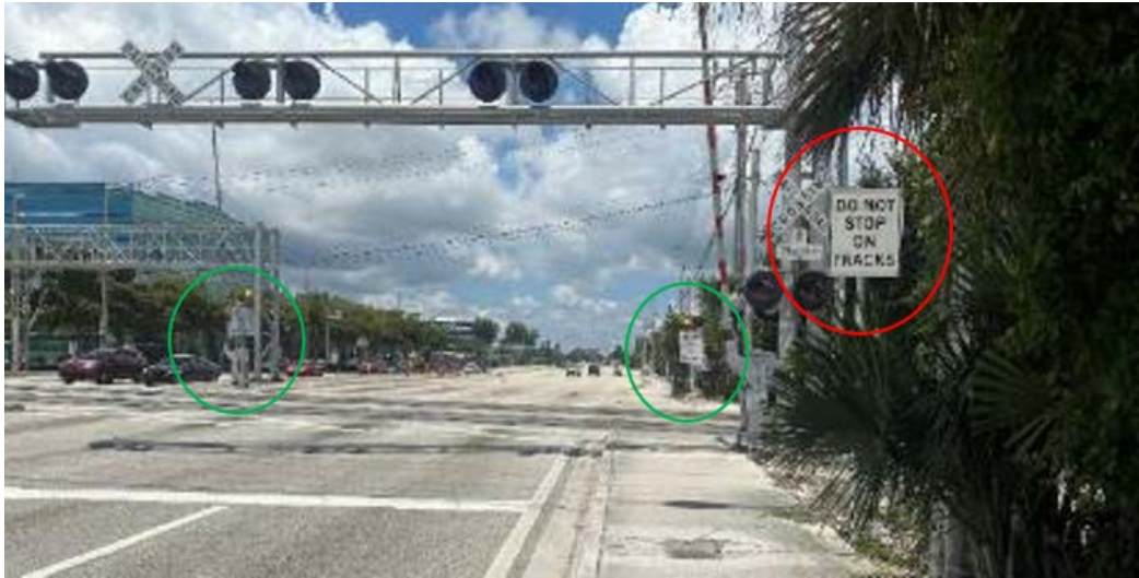
Figure 6-22. Signs with Flashing Lights on WB Median at W Cypress Creek Rd @ N Andrews Ave, District 4
