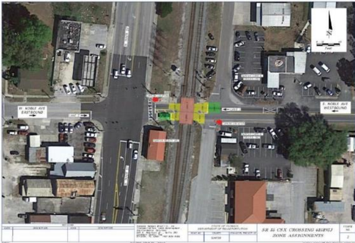
Figure 3-7. Positioning of the Cameras at an HRGC to Collect Driver’s Stopping Behaviors
