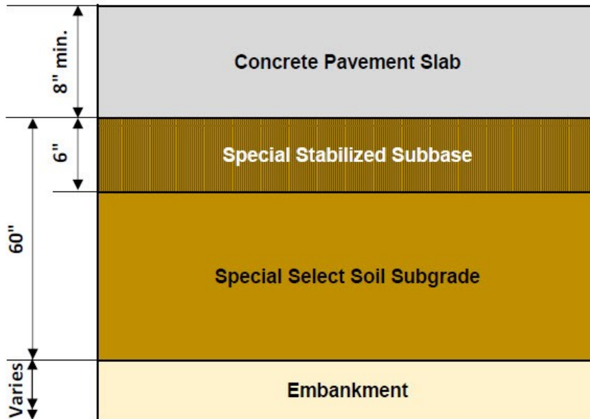
FIGURE 2.2 SPECIAL SELECT SOIL BASE OPTION
