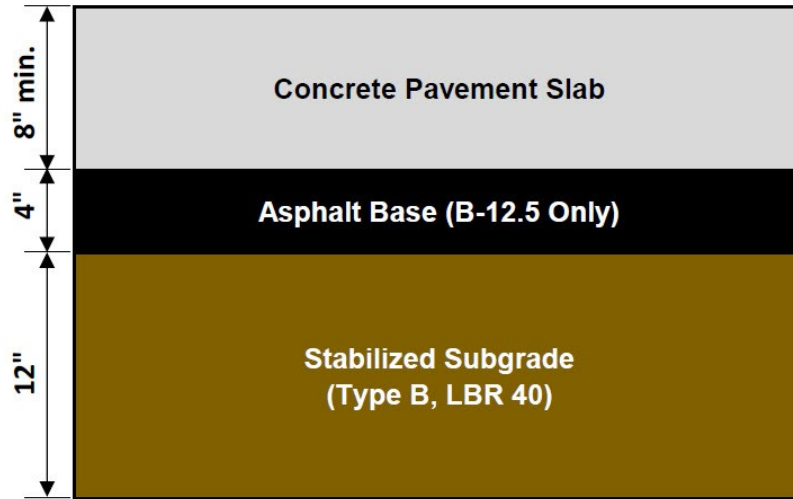
FIGURE 2.2 SPECIAL SELECT SOIL BASE OPTION
