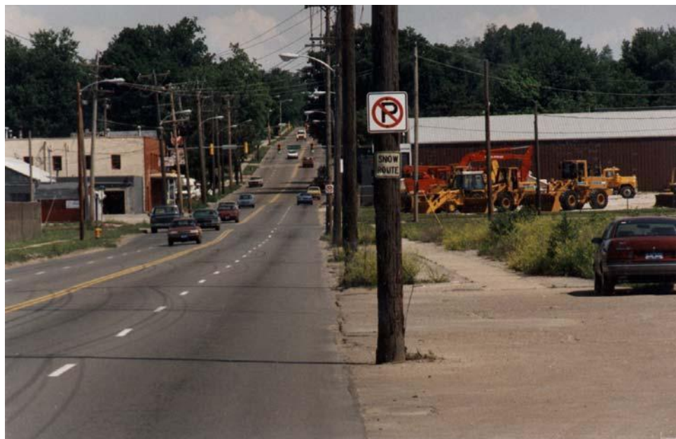
FIGURE 25 Lateral offset to obstruction is an operational offset and is not the same as clear zone.
