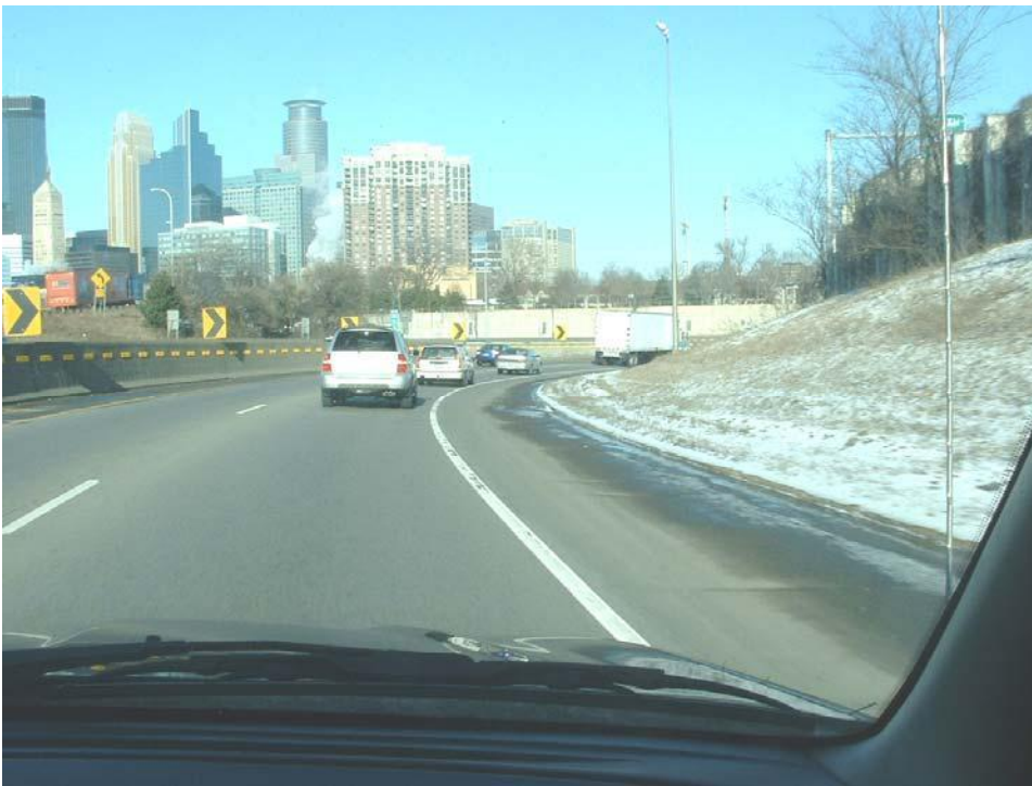
FIGURE 50 Delineation with large chevrons.
