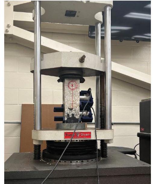
Testing setup for small-scale 50-kHz and 500-kHz testing on block specimens.
