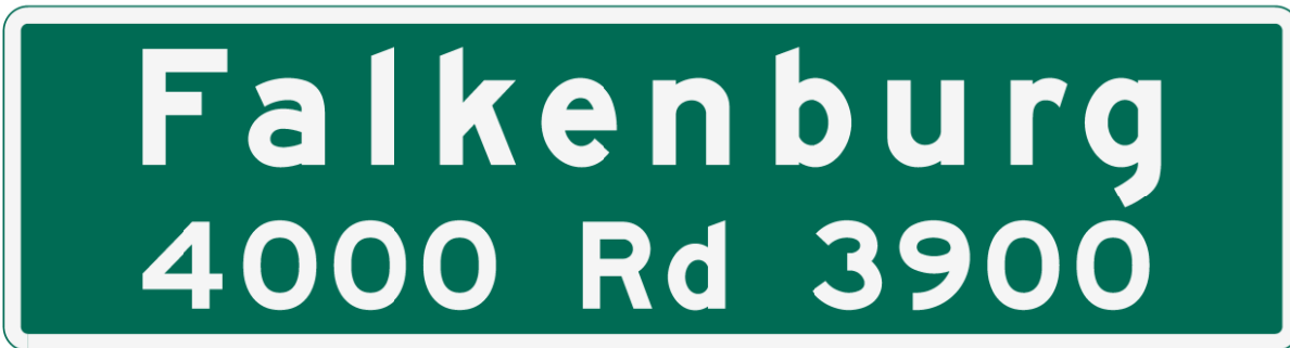
Figure 2.2-1. Overhead Street Name Sign
