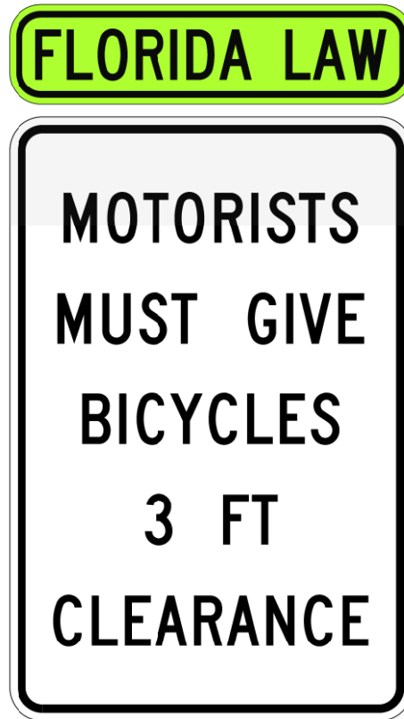
Figure 2.11-1 Bicycle Passing Clearance Sign
