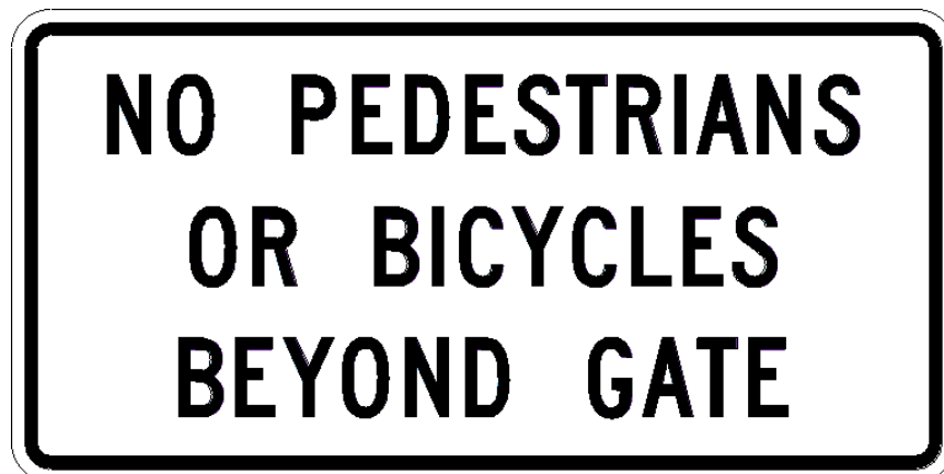
Figure 2.6-1. Swing-Style Pedestrian Gate Sign on Movable Bridges
