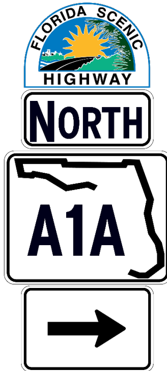
Figure 2.34-3. Co-location on Route Directional Marker
