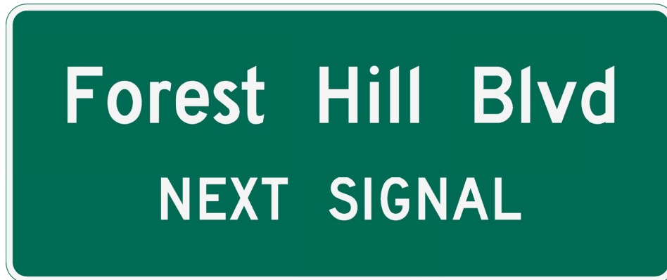
Figure 2.37-2. Advance Street Name Sign Design (Single Post)
