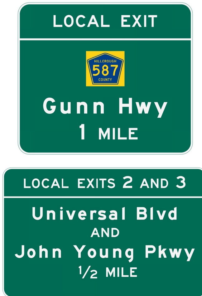
Figure 2.42-6. Examples of Egress Signing
