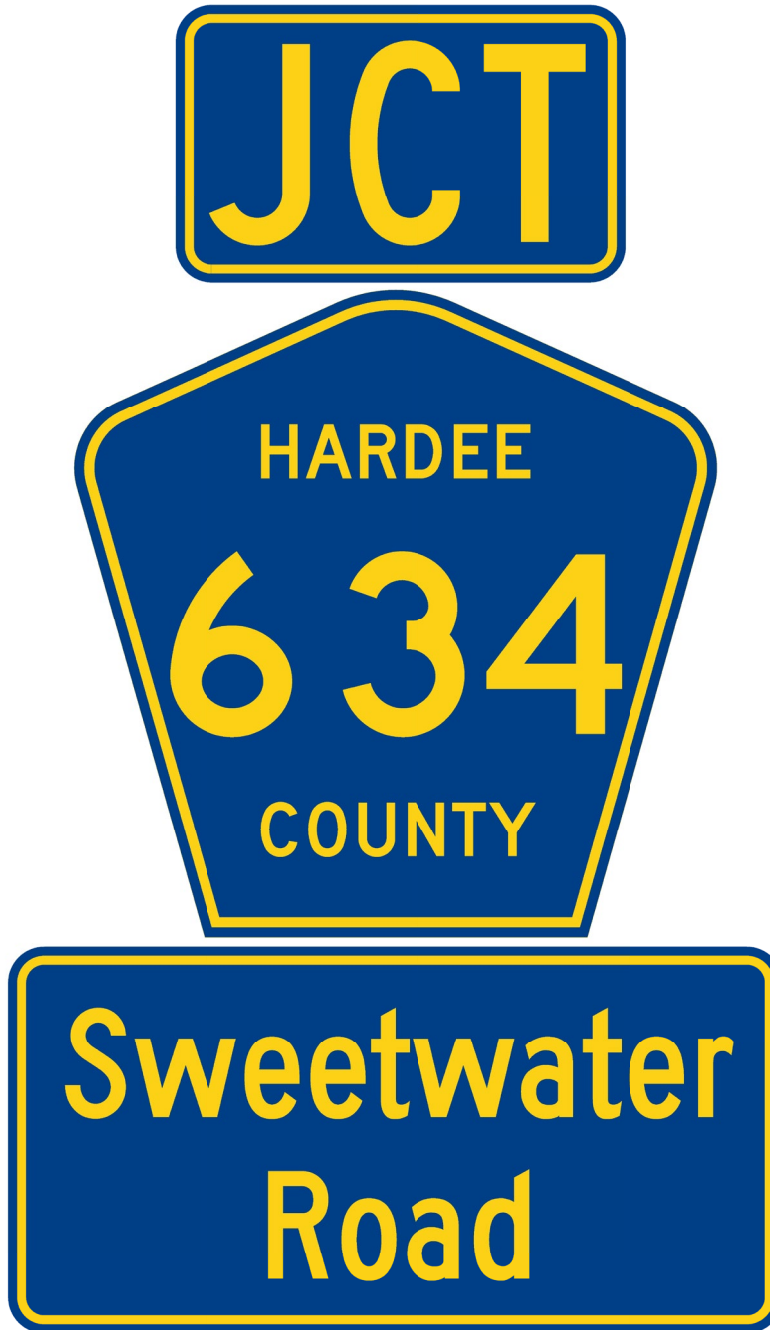
Figure 2.37-9. Advance Street Name Plaque on Advance Route Marker
