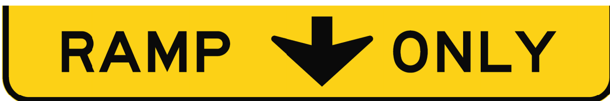
Figure 2.43-1. RAMP ONLY Sign Panel
