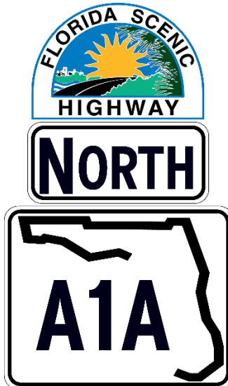
Figure 2.34-2. Co-Location on Route Confirmation Marker
