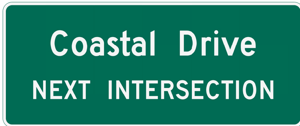
Figure 2.37-6. Advance Street Name Signs at Non-Signalized Locations
