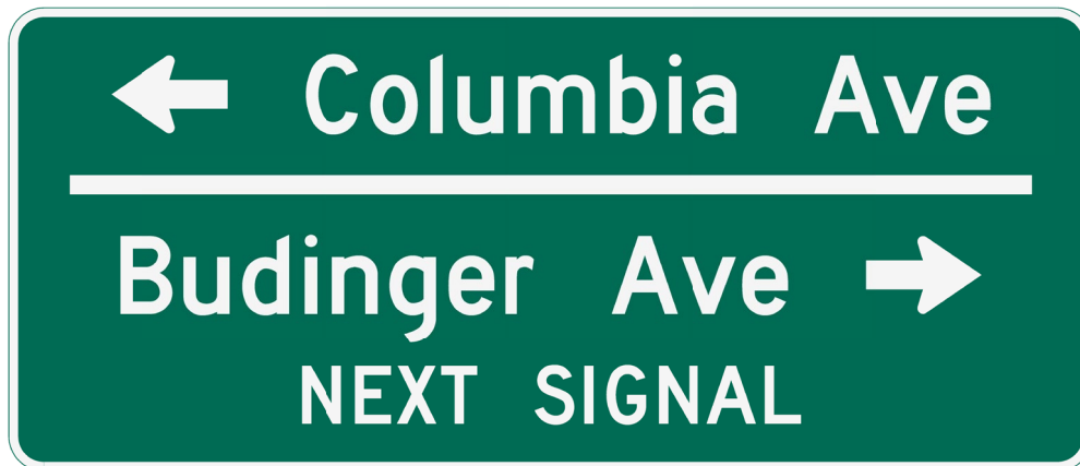
Figure 2.37-5. Advance Street Name Sign Using Different Names
