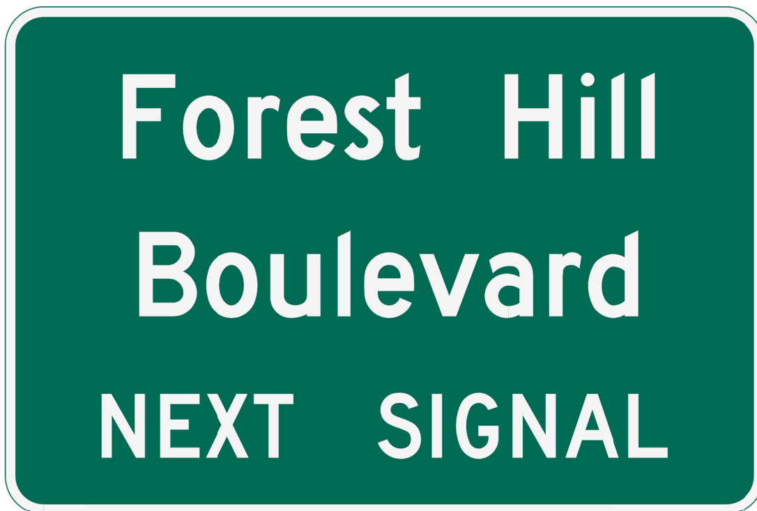
Figure 2.37-3. Advance Street Name Sign Design (Double Post)
